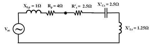
Then, combination of the primary impedance and the total reflected secondary impedance would result in the equivalent impedance  $\mathbf{Z}_{eq}$ :
