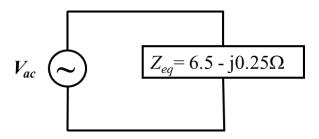
The equivalent impedance  $Z_{eq}$ , derived in the rectangular form above, can be stated in polar or phasor form as:
